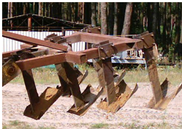
Fig. 1. Working equipment for deep continuous cultivation of the soil with improved racks
